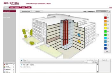
Building view: humidity
